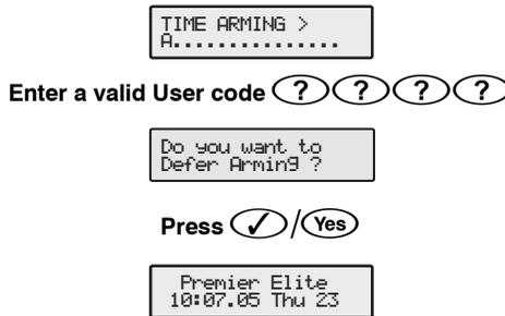
The system will return to Time/Date displayed on the keypad and defer Time Arming of the system, for example by 30 mins, or whatever has been programmed as the defer arming time.
